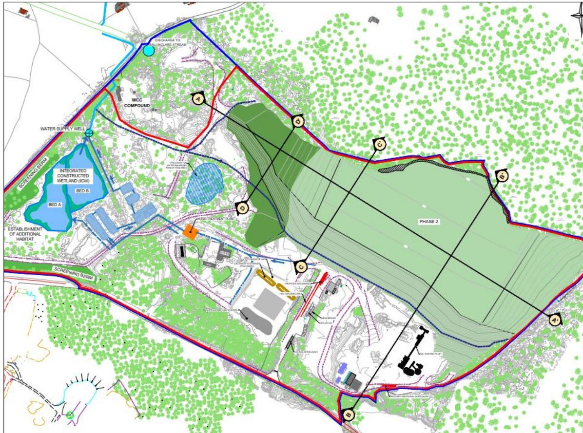
Landfill raised to 80mOD with section of existing quarry face (up to 15m high) remaining exposed
